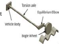
The suspension structure of modern tank torsion axle
