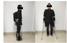
Lower Exoskeleton Robot Driven by The Series Elastic Actuator
