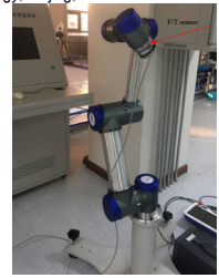
The 6-DOF manipulator IRIC-I developed in our laboratory
