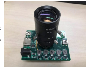
High-speed Vision Detection System Based on FPGA
