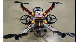
A Quadrotor with Auxiliary Thrusters
