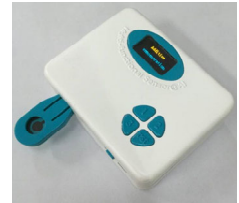
Portable Wireless Food Safety Rapid Detection Device
