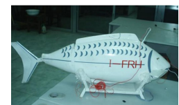
The prototype of robotic tuna
