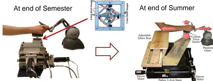
Started with bench-top Shear feedback device. Added custom force sensor and controller. Ongoing PhD research for Mark Fehlberg
