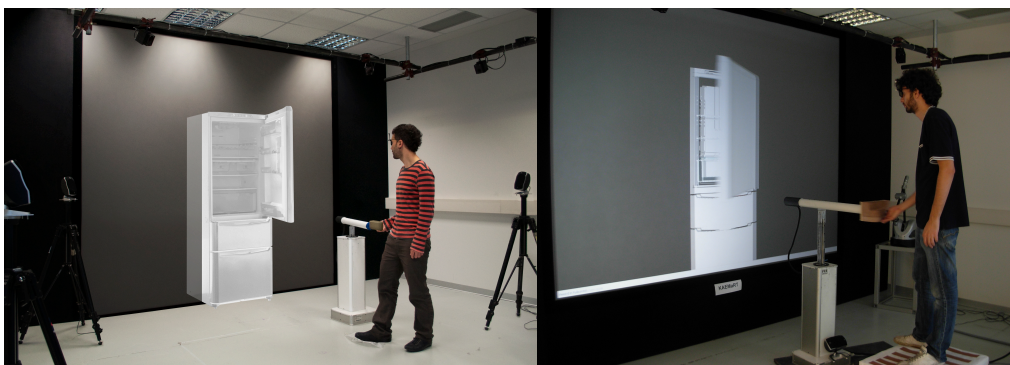
Figure 2. During the second phase of the research activity we have simulated the interaction with a commercial refrigerator. The haptic interaction is improved thanks to the use of a milled prototype of the handling attached to the end effector of the haptic device.
