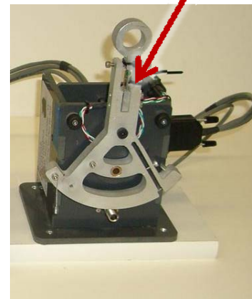
Utah Haptic Paddle PVC base, aluminum handle with integrated force sensor (M. Rasmussen, M. Fehlberg, A. Doxon, W. Provancher)
