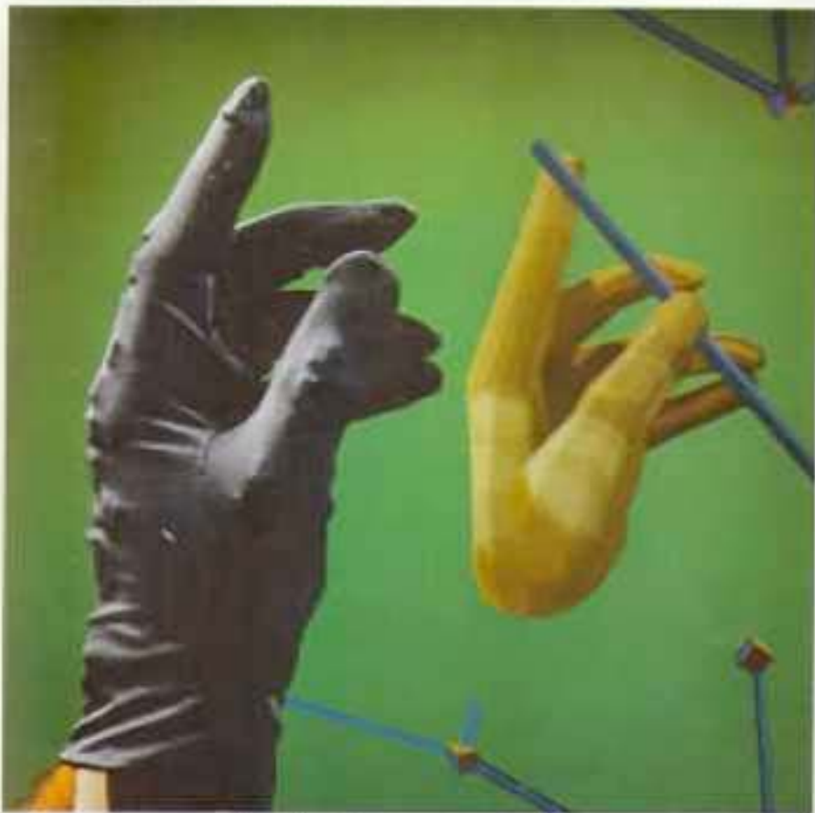
Wiref Glove gives a computer user the sensation of handling objects on the screen; the image of the hand mimics the user's movements.
