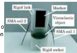
Loosely coupled joint driven by SMA Coils
