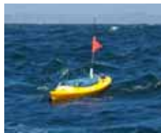
An autonomous kayak performing adaptive sampling in Monterey Bay, CA
