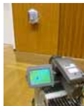
An alterable thermo landmark and a mobile robot with IR camera.
