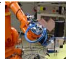
Force-controlled drilling using an ABB Irb 2400 industrial robot
