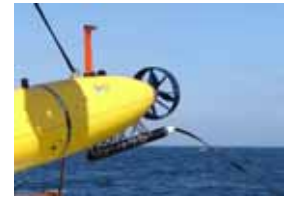
The MIT vehicle with the towed vector sensor array
