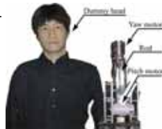
An acoustical telepresence robot: TeleHead and its inside.
