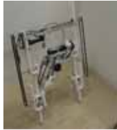
A four link biped with shank and thigh in each leg. The knee joint has a stopper to avoid hyper-extension and latches to lock the joint.
