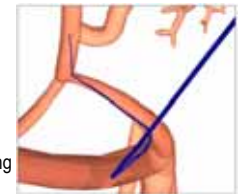
Motion planning of a 2,500-DOF articulated chain as a catheter in a network of arteries
