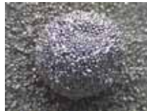
Pattern made with a water drop covered with nickel fillings.
