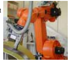
Industrial sewing robot with blindstitching head.
