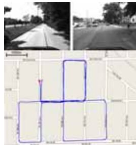
Experimental results: 10m position error after 3.2km trajectory in urban environment
