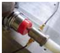
Actuation of a push-button switch using an instrumented probe
