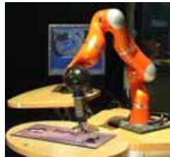
DLR-KUKA light-weight robot inserts planar parts automatically using vision and impedance control.
