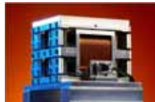
A prototype of Flexure-Based Electromagnetic Linear Actuator (FELA)
