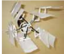
Flying Robot with Pantograph-based variable wing Mechanism
