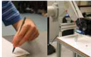
Humans use bracing to increase precision during fine manipulation tasks. It is known that bracing improves manipulator precision as well.
