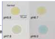
pH sensing gel-tool for local pH measurement
