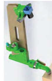
CAD model of the Proton 1, shown with the OptoForce end-effector contacting a surface.
