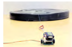
A \mu Tug micro-robot with integrated tactile sensing is able to maximize its pulling capability using force feedback.
