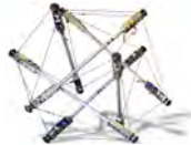
The SUPERball tensegrity robot. We learn a rolling gait from scratch for this robot with our algorithm.
