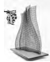
Mesh Mould Metal End-effector and fabricated mesh
