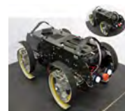
The leg-wheel transformable robot TurboQuad .
