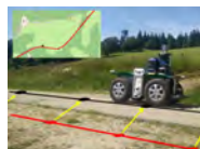
Our approach aligns subgoals from OSM (red) with the street, classified from 3d-lidar data (black).
