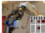
Tactile feedback is exploited for contact modeling.
