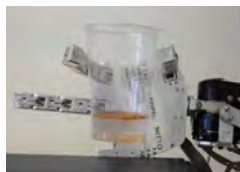
The tactile sensor mounted on the fingers of the Vizzy robot hand.
