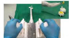
Manipulator system with a purely mechanical control concept
