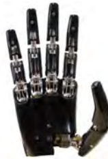
Robot Hand based on TSA mechanism
