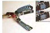
Tunable friction pads attached to the fingertips of a soft robotic gripper.
