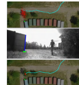
FLAG updates global position by matching large vertical features from the ground to features in an aerial image
