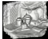
Dense reconstruction of an office desk obtained using the normal-based prior
