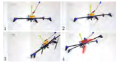
A tilted-propeller hexarotor recovering from a failure thanks to the analysis and the controller proposed in the paper.
