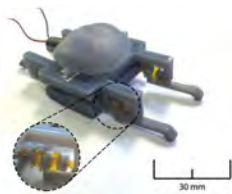
A 30 mm long, 6 g millirobot made with 3D printed rigid components and Kapton flexures
