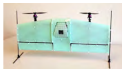
The IDSC Tailsitter. This vehicle is used for experimental validation of the proposed controller.
