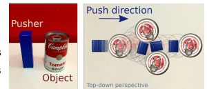
A quasi-static pushing problem: the pusher has a velocity controller with low gain, resulting in non-Gaussian transitions.
