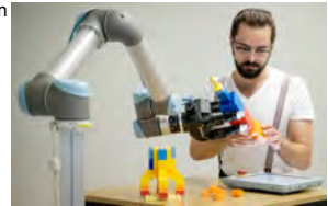
In a collaborative Lego assembly task, the robotic assistant continuously coordinates its behavior with the human co-worker.
