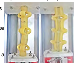
Passive return mechanism : slit mechanism (right) | Telescopic mechanism (left)
