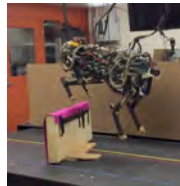
Proprioceptive actuators provide impact mitigation for dynamic locomotion
