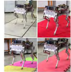
The quadruped robot Biodog locomotes on different ground substrates in walk gait.
