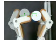
Vision-based within-hand precision manipulation with Model T42 hand.
