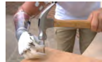
Our four-bar linkage driven-finger is compliant and resistant to impacts from multiple directions.
