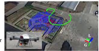
This system allows a UAV to localize accurately within a geo-referenced map that is built during a reconnaissance flight
