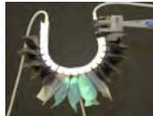
Figure: An inflated actuator featuring a heterogeneous bending profile.
