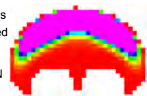
Fig. 1: Reachable space of a Dubin's car robot with max speed constraint. Color spectrum correlated to number of graph states.
