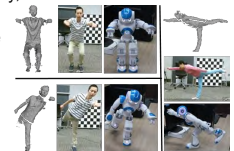
Three different poses retargeted to NAO robot using our proposed approach. The mesh and color image are captured by Kinect V2.
