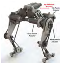
MIT Little HERMES: robot designed for balance experiments during full body teleoperation.
