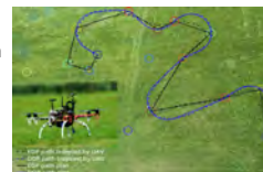
Real experiment with hexarotor UAV of VNS-based method for the Dubins Orienteering Problem
