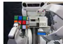
The robot is able to precisely manipulate the Rubik's cube using the equipped pre-touch sensors.
