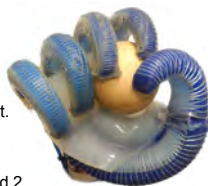
The sensorized RBO Hand 2 performs a compliant grasp
