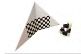
The calibration system incorporating a calibration target (formed by two triangular boards with a checkerboard on each one) and a capture rig (consisting of a 2D LRF and stereo cameras)
