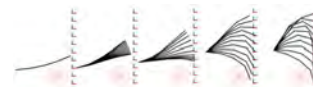
Iterations in an optimization to find the best base position and subsequent arm motion for a linear trajectory
