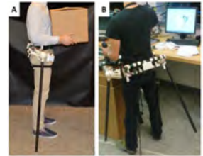
A. Prototype of the additional robotic limbs. B. Human subject controlling the robotic limbs with torso EMG signals.
