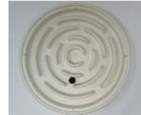
A circular maze is mounted in a in-house tip-tilt platform. The goal is to learn a control law to drive the ball to the center.
