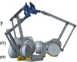
CAD model of the (6+3)-dof hybrid parallel robot including partial static balancing
