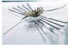
The miniature water-walking designed to study the flexible driving mechanism
