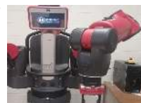
7-DoF redundant manipulator with offsets at shoulder, elbow and wrist joints
