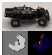
A mini race car (top) explores a 2D environment (bottom left) based on the mutual information map (bottom right)
