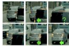
Left turn (←) and occlusion (?) correctly classified in video sequence
