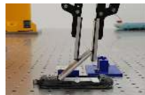
Shallow-depth insertion demonstrated through phone battery insertion.
