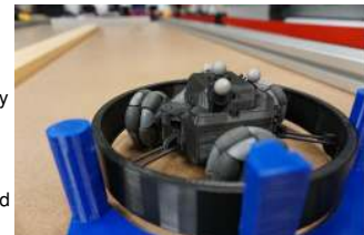
Equipped with a protective, collision-energy restoring ring; Omnipuck awaits launch in a 3D printed jig before each experiment.
