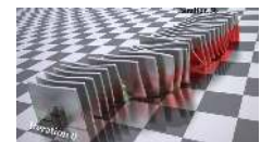
Bottom to top: learning to walk in only 58 gradient descent iterations using our differentiable simulator.
