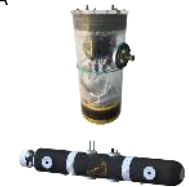
Single degree of freedom test cylinder (top) and CephaloBot AUV (bottom).
