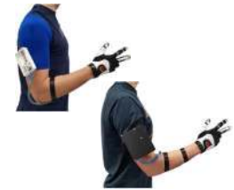
Side view of the proposed exo-gloves: body-powered (top) and motorized (bottom).
