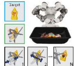
The system selects between grasping and pushing objects until the target object is extracted.
