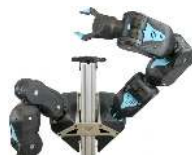
Blue, a 7-DoF Quasi-Direct Drive robot arm
