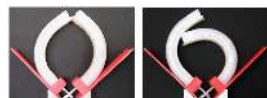
A two-fingered gripper exhibits different behaviors depending on the actuation rate from a single pneumatic line.
