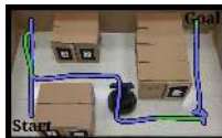
Novel Belief-Infused FSC is in the controller family; blue are FSC nodes, and green are belief points
