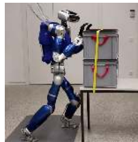
TORO pushing a table with a weight of 50 kg on top
