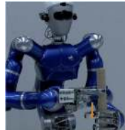
Tactile material classification by sweeping a finger over an object's surface.
