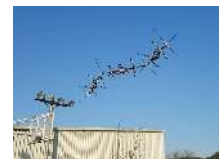
Outdoor flight experiment of 3-link aerial skeleton system
