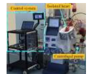
Automated aortic pressure control system for ex vivo heart perfusion
