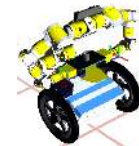
A wheeled inverted pendulum humanoid carrying a cup on a tray
