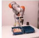
Setup for learning the skill of grasping objects from a densely filled bin
