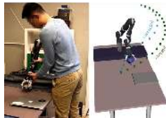
The user provides a correction to the green trajectory. The blue trajectory shows one possible interpretation of the correction.
