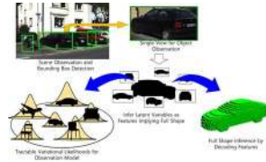
Fig. 1. In order to approximate the object observation model, we train the variational auto-encoder to achieve the object generative model.
