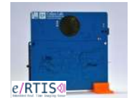
A 3D imaging sonar sensor using a pseudo random microphone array
