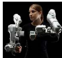
Harmony is a bimanual upper-body exoskeleton designed to actively control 7 DOF
