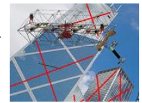
Aerial platform with suction-based gripper for performing lateral work.
