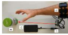
System schematic. As the user reaches for the desired object (a), the forearm-mounted RGB-D video camera (b) and Myo armband (c) stream data to a smartphone application (d).
