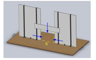
FIGURE 3: WALL TILE. BY MOVING THE PANELS, THE APERTURE WILL BE REDUCED TO MATCH ROBOT DIMENSIONS.
