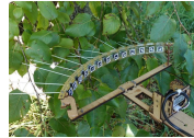
The system comprises soft artificial whiskers with fiducial markers and a camera
