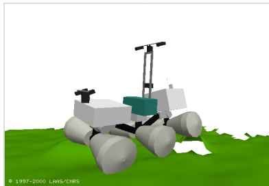
Convolution of the robot model with the terrain model
