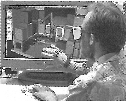
Fig. 16 Two handed VR-interface using Space Mouse and Data Glove (space station scenario as example)
