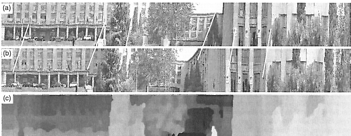
Fig. 10. (a), (b) Omnistereo pair and (c) the depth map of the Main Building at Tsinghua University from a ground vehicle video sequence (1024 frames of 128*128 gray scale images).
