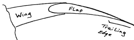
Figure 1: Concept of a variable camber wing
