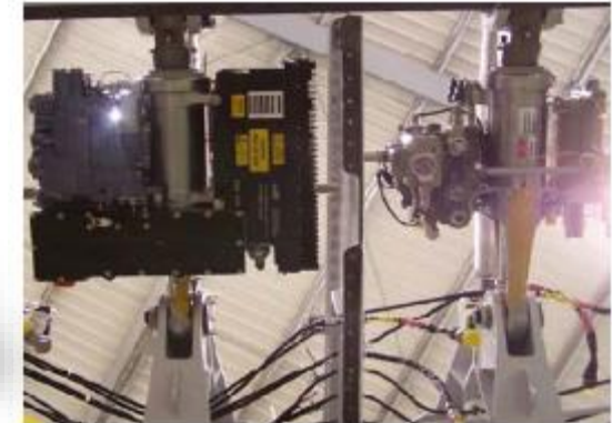
Two adjacent dissimilar actuators for moving a single control surface on the A380 On the left: an EHA, and on the right a conventional hydraulic actuator.
