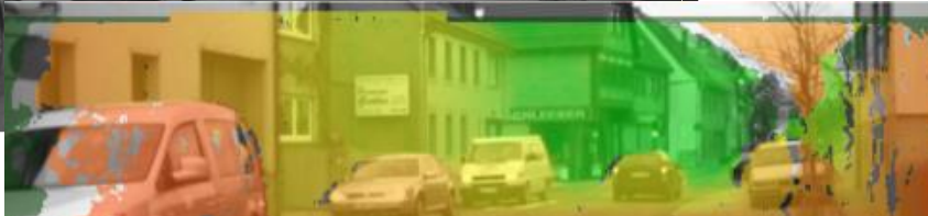
Disparity Image (SGM) 500.000 points in 3D real-time on FPGA
